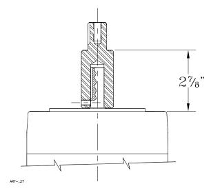
**Checking pump shaft run -out:** Place the motor with the shaft facing up. Attach a dial indicator with a magnetic base or clamp with a plate bolted to the motor (as shown). Place the dial indicator on the end of the shaft and rotate the shaft. The Total Indicated Run out (TIR) should be no greater than .004".
