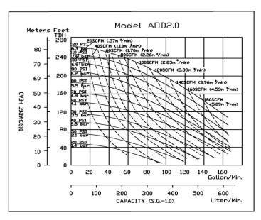
The performance curves shown and other published literature reflect an average performance for all materials and all elastomers, including Teflon®. Derating of the performance is not necessary for Teflon® fitted pumps.
