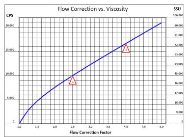
To determine the correction flow rate, find the intersection of the VISCOSITY on the above curve and read the FLOW CORRECTION FACTOR. Multiply this factor by the desired flow of the pump and use this new flow rate to select a pump from the performance curves.
